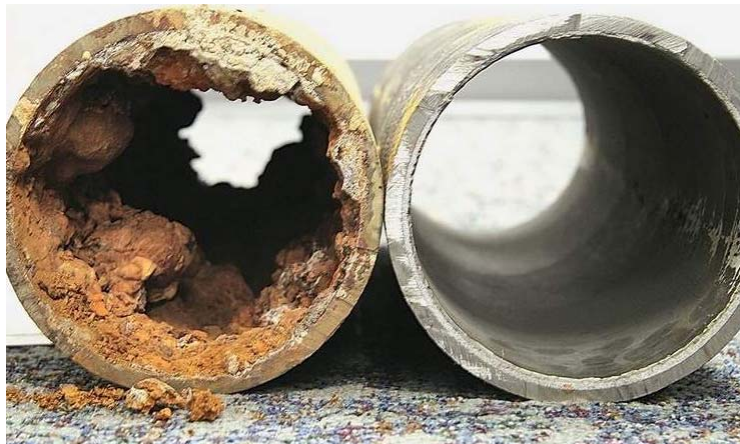
Tuberculation in the water main system City of Rockville
